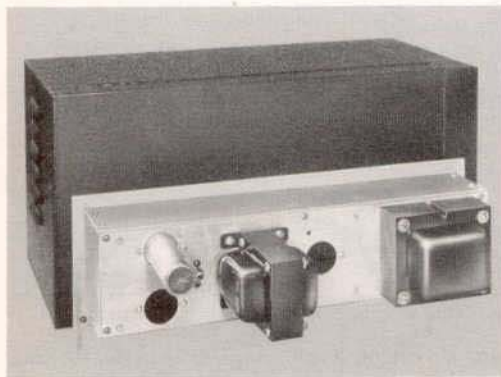
REAR VIEW of a table cabinet model GADGET RACK with power supply fastened to rear wall. Slot across rear of cabinet provides access to interconnection sockets from inside cabinet.
